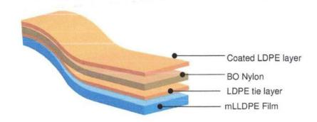
CNL 75 - is manufactured through the process of Extrusion Lamination
